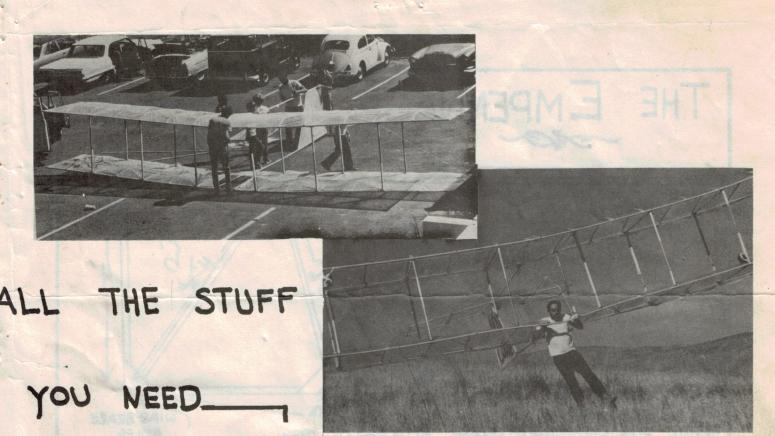
THEN GET 2 16' BAMBOO POLES 2" DIA. CUT 2,4'3" LENGTHS FOR ARMPIT HOLDER ALSO CUT THE REST INTO 4'6" CHUNKS SPLIT FOUR TIMES INTO 21 RIBS (SEE DETAIL) 96 4" TRIANGULAR CAROBOARD, GUSSETS \_ 24 POLE HOLDERS (CLOTHES CLOSET TYPE) 25 YARDS 10' WIDE PLASTIC SHEET 2" X I'XI" ALUMINUM ANGLES 66 WOOD SCREWS 21 2" X 32 EYEBOLTS CONSTRUCTION PAPER O-man Br 300' BAILING WIRE BALL HEAVY STRING RIBSTITCHINGS SOZ WHITE GLUE 200 STAPLES ROLL I" MASKING TAPE PLUS PATIENCE, A FRIEND, HILLS, SUNSHINE,
