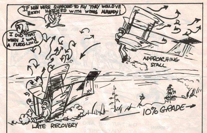
IF THE MACHINE SEEMS TO STOP IN THE AIR AFTER CLIMBING A BIT, YOU ARE STALLING.... MOVE YOUR LEGS FOWARD TO ANGLE DOWN AND PICK UP SPEED.
